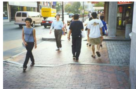
Sidewalk paving should be carried over across any intervening driveway.
